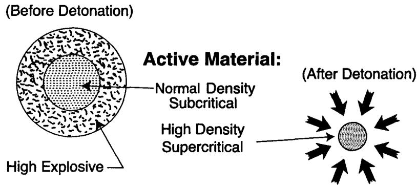
Figure 2-VIII. Implosion Assembly Principle
