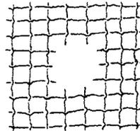
3. Put the grid in the pit. Bend the ends of the wires, or put a small stone at each corner, so that the grid stands about 3 cm. off the ground.
