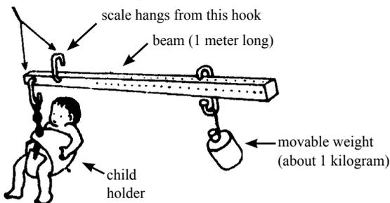
Weight is correct when beam stays horizontal.
