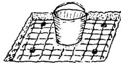
5. Mix cement with sand, gravel, and water and pour it until it is about 5 cm. thick. (With each shovel of cement mix 2 shovels of sand and 3 shovels of gravel.)
