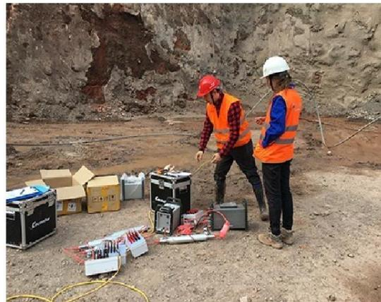
GD-20 is portable and equipped with internal storage for data recording. Multichannel switch box. GD-20 is capable of performing VES, ERT and For VES, 12 depths can be measured concurrently. For ERT surveys, data acquisition can record up to 10 concurrent channels. mode satisfies the need for arrays with infinite far electrodes of N terminal, with 10 individual acquisition channel for the best data collection efficiency.
