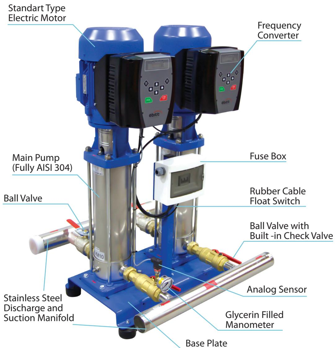
**Automatic Water Boosters with Frequency Converted Pump Units
