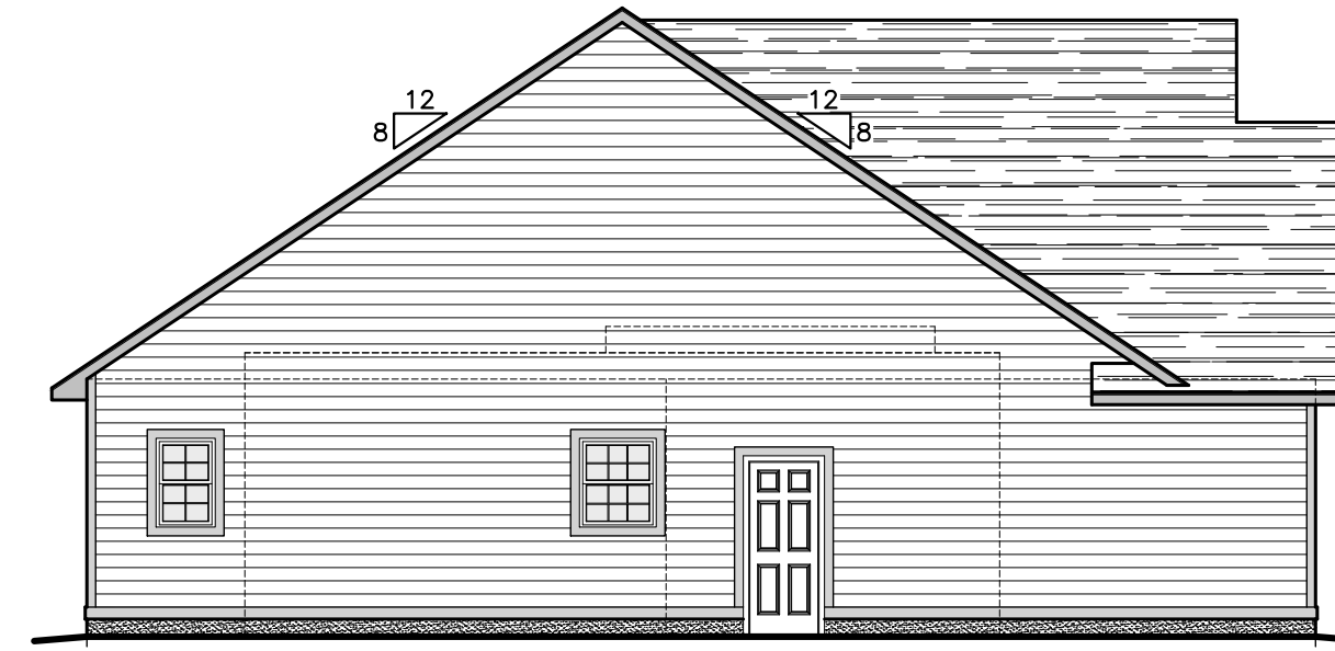
2 3 LEFT SIDE ELEVATION SCALE: 1/8"=1'-0"
