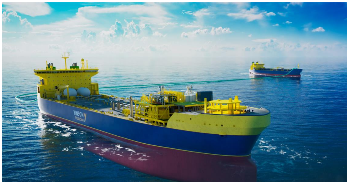
An illustration of a FSIU in the foreground, receiving cargo from a LCO2 carrier in the background.
