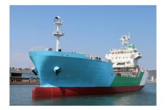
LNG cargo tank capacity: 3,500 m<sup>3</sup> Gross tonnage: 4,100 tons Length overall: 81.7 m Breadth: 18.0 m Delivery: September 2020 Shipyard: Kawasaki Heavy Industries Ltd., Sakaide Works
