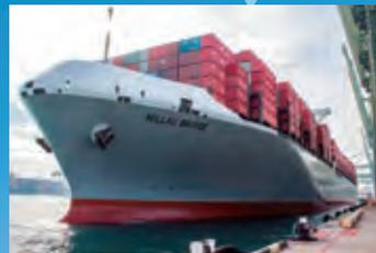
The super-sized (14,000TEU) container vessel *MILLAU BRIDGE* with the latest energy-saving technologies was completed.
