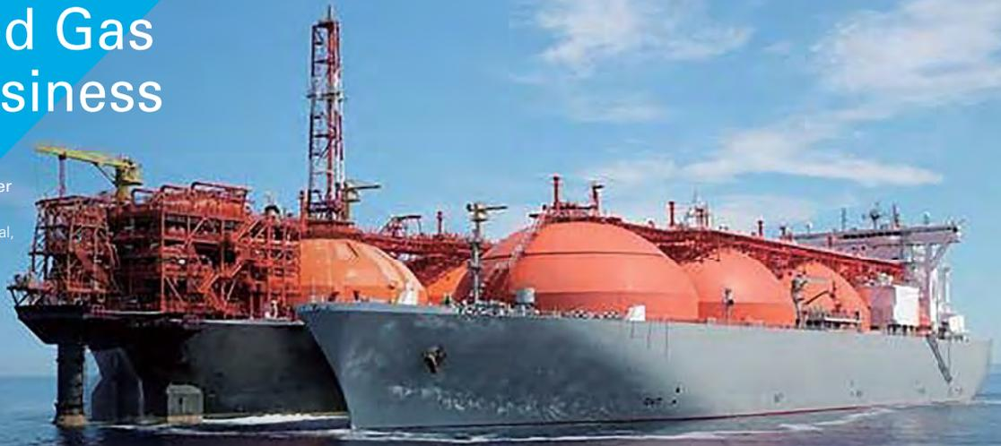
Floating Storage and Regasification Unit (FSRU) for LNG
