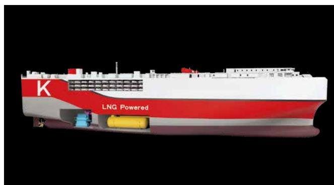
LNG-fueled car carrier conceptual drawing
