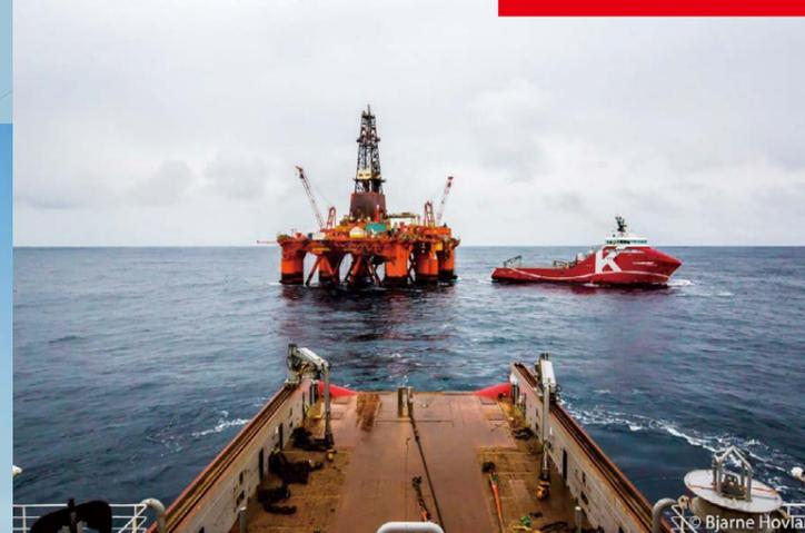
Anchor handling tug supply vessel performing a rig move
