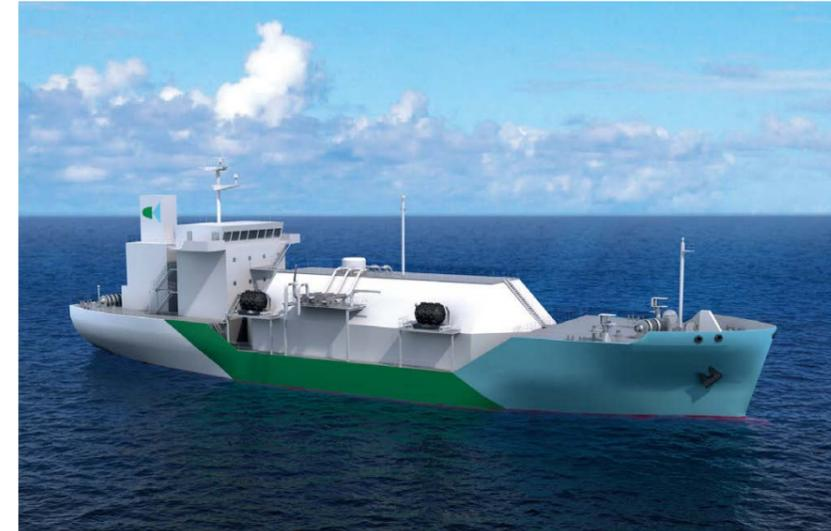
LNG bunkering vessel Photo: Kawasaki Heavy Industries, Ltd.
