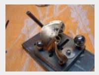
\*\*\*\* Special Note: When cupping ANY prop, startip or round ear...the ramping on the trailing edge of the prop MUST be removed prior to pounding it on the block. (The ramping only needs to be removed for the distance the ball will be in contact with the trailing edge.)
