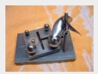
Above is a mock up of what a blade will look like if it's bent. It will either fall forward or behind the pen mark. (You may need to fool around with all the blades to find the one that is correct, then mark the ball and proceed checking from there.)
