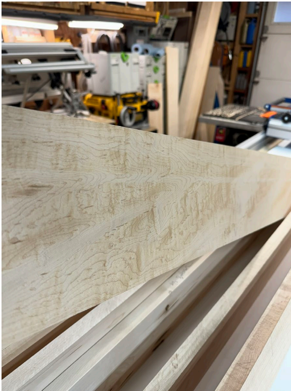
Near curly maple grain figuration (creates a sense of depth when finished)
