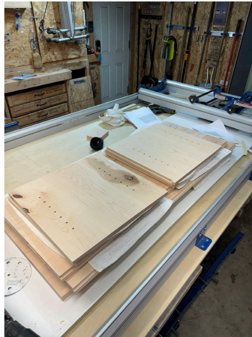
Details cut including inset for rear panel bottom side reveal and pin holes for adjustable shelves
