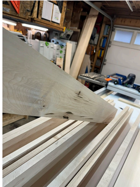
Interesting grain interruptions in just one or two boards (these are not knots)
