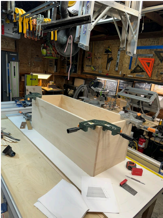
Checking square, fit and marking detail cuts/punches to be made prior to final assembly
