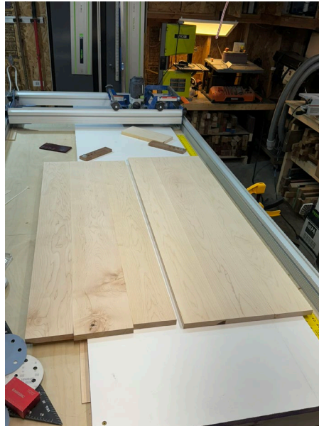
Joined panels with first sanding pass complete. Intentionally long for cutting post-join to spec.
