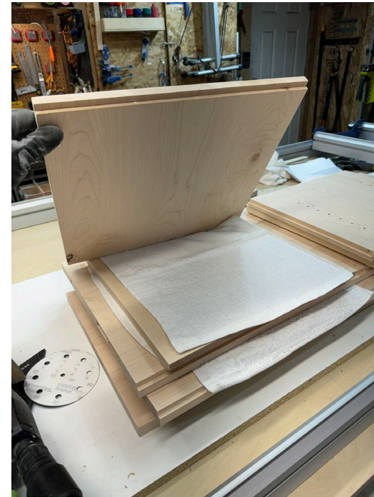
Each panel is sanded to 220 grit pre-assembly, making post glue-up finishing much easier
