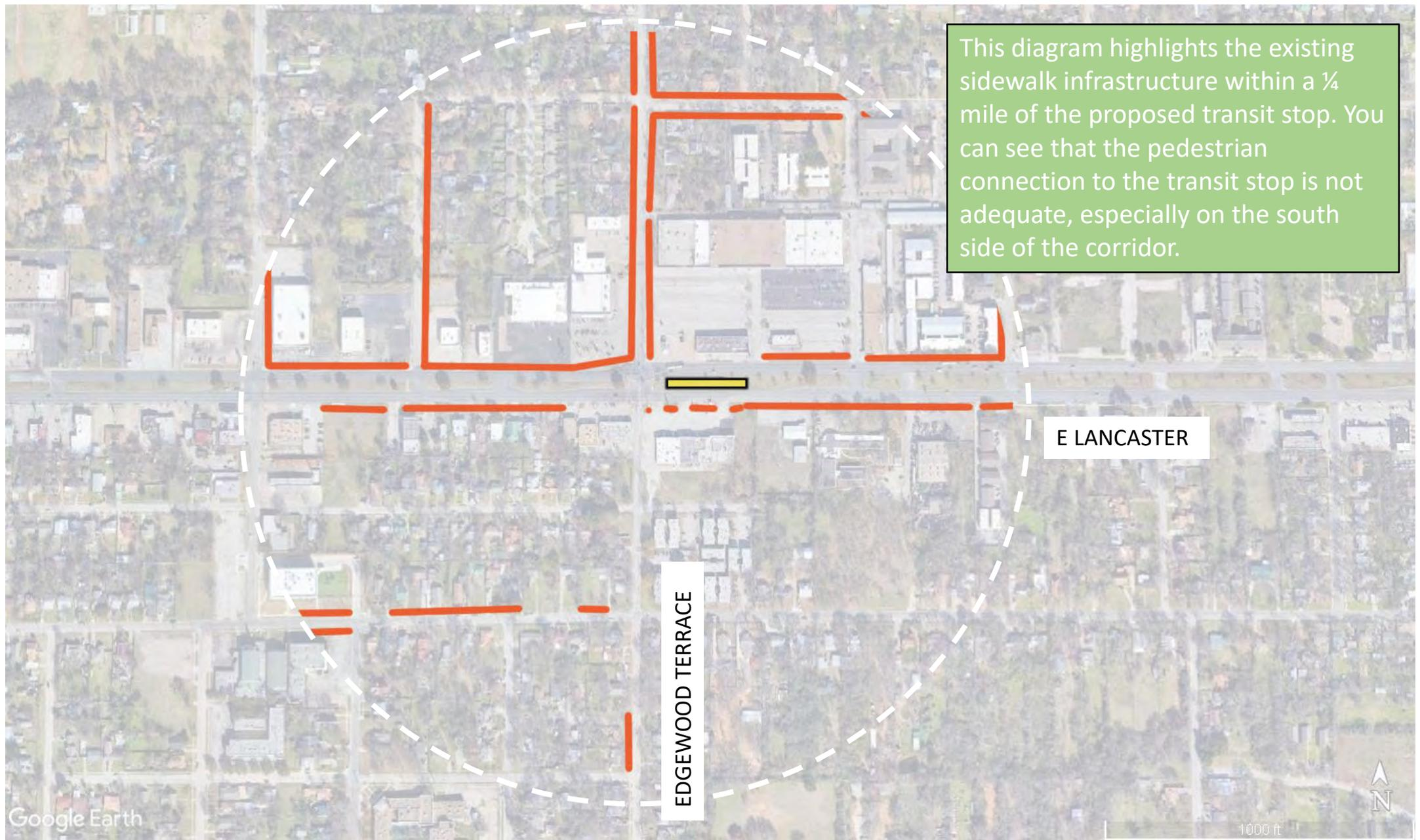
This diagram highlights the existing sidewalk infrastructure within a ¼ mile of the proposed transit stop. You can see that the pedestrian connection to the transit stop is not adequate, especially on the south side of the corridor.
