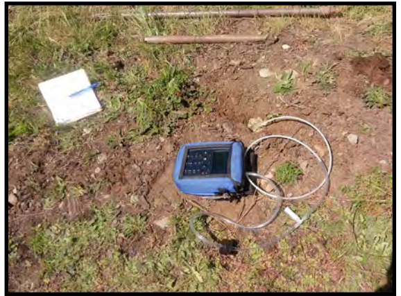
Performance of Landfill Gas survey through borehole sealed at surface.
