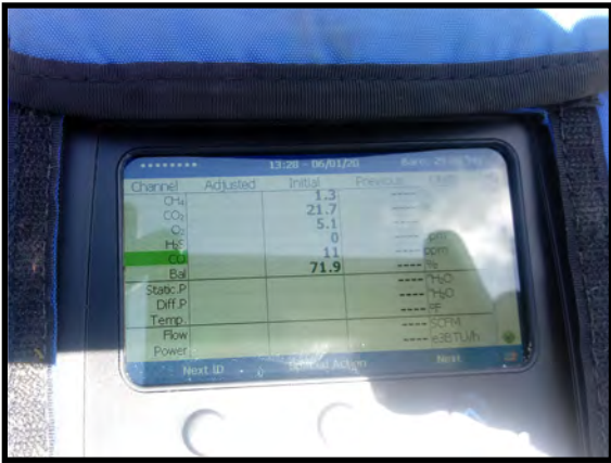
Landfill Gas reading; GEM 5000 instrument
