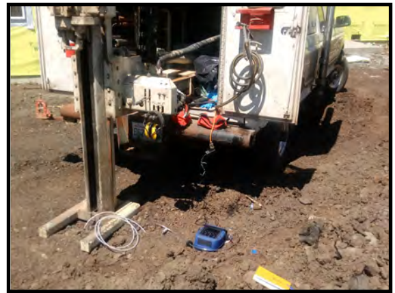
Collecting Landfill Gas reading through polyethylene tubing inserted into a sealed borehole.
