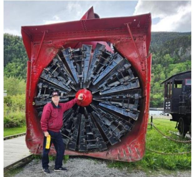
Annual snowfalls of over 20 feet often brought rail traffic to a halt. Until 1964, White Pass & Yukon Route maintained a fleet of rotary snow plows used to keep the vital link of rail open. Experienced rotary operators worked with pusher engines to clear the track, often churning through drifts higher than the engines themselves. The workers communicated using a series of whistles signaling stop, back up and forward.
