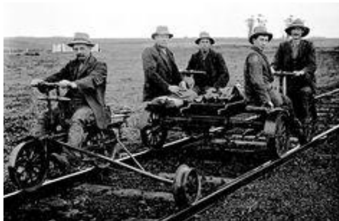
Left: Pedal powered Velocipede. Heavy metal and railway wheels made it possible to stay on the tracks.
