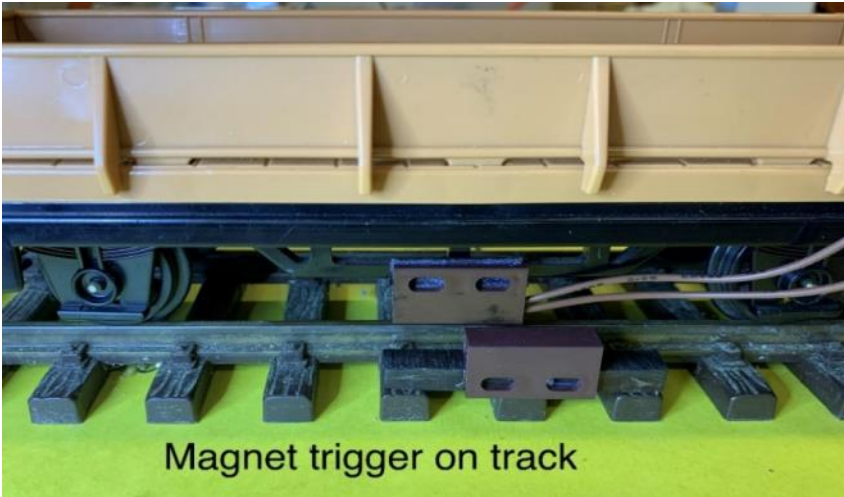
Figure 5 Magnet Trigger on Track beneath Magnetic Switch
