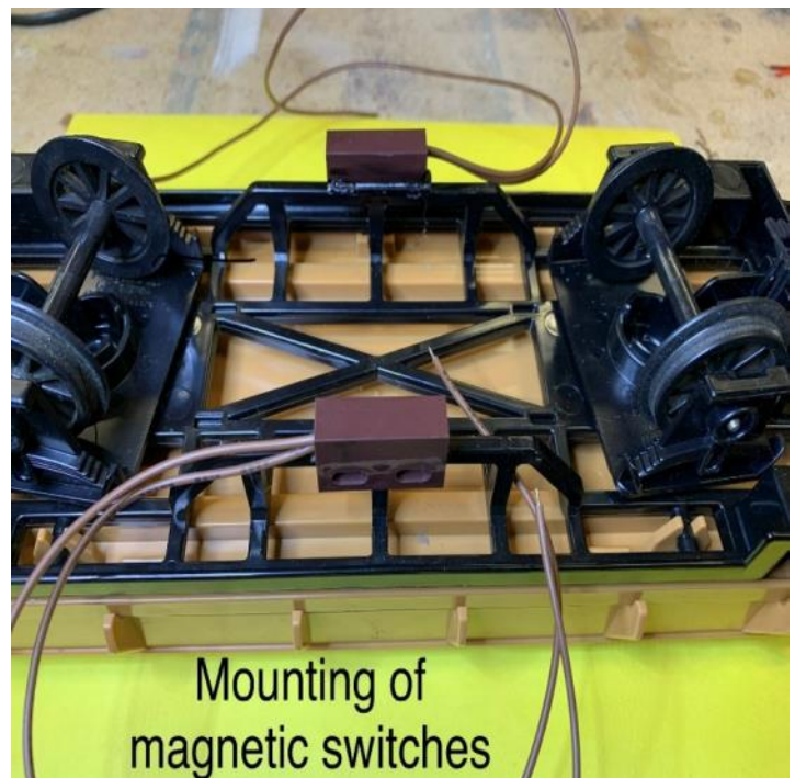
Figure 4. Magnetic switches underneath flat car
