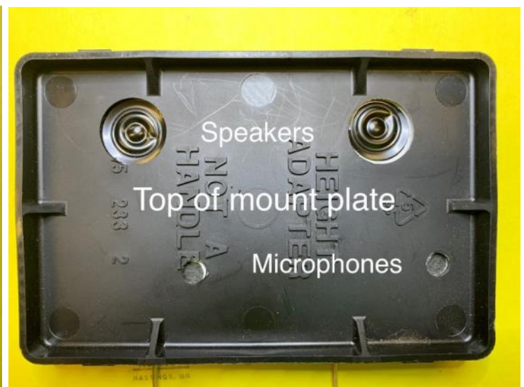
Figure 7 Top of Sound Module Assy
