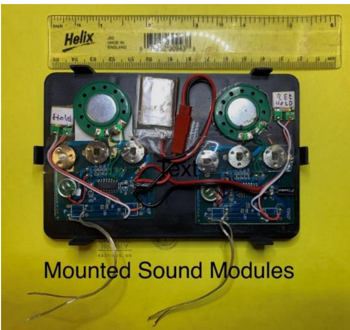
Figure 6 Two Sound Modules fastened to Plastic Panel
