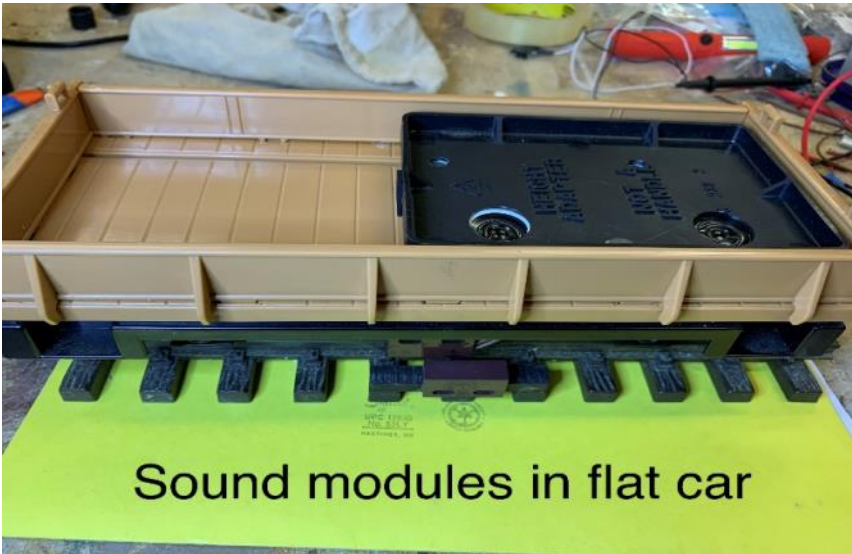
Figure 9. Completed Sound Flat Car
