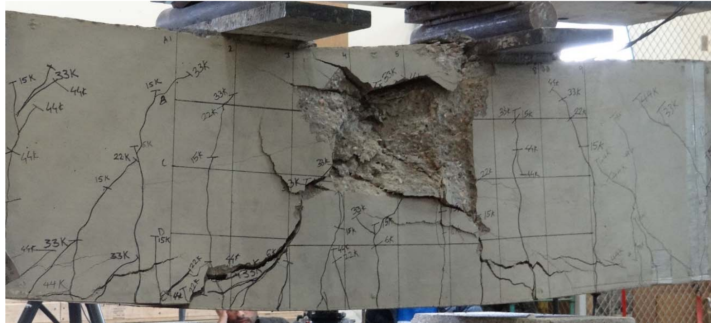
RC #2 beam (Plain Concrete + BFRP bar)
