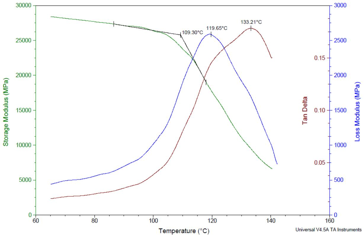
Figure 3.2 – Storage modulus / loss modulus vs temperature response graph for a representative test.
