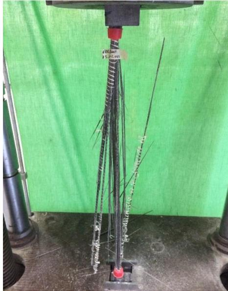
Figure 5.3 – Representative failure mode of tensile test
