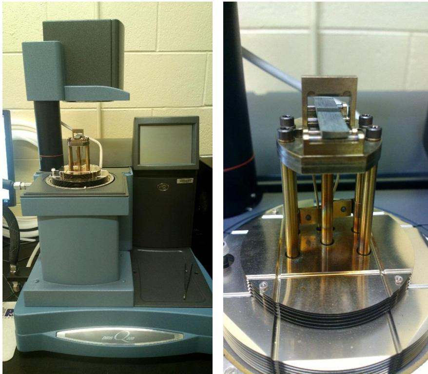
Figure 3.1 –  $T_g$  test set-up
