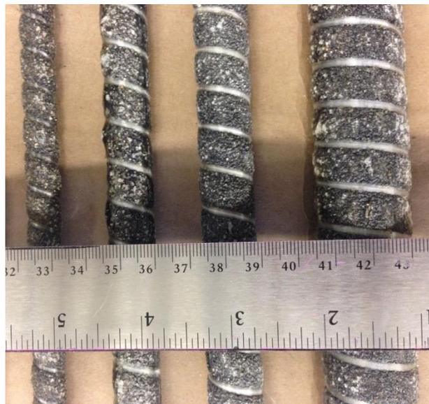
Figure 1 – RockRebar™ Basalt Fiber-Reinforced Polymer (BFRP) composite reinforcing bar under evaluation, from left to right #3, #4, #5 and #8.
