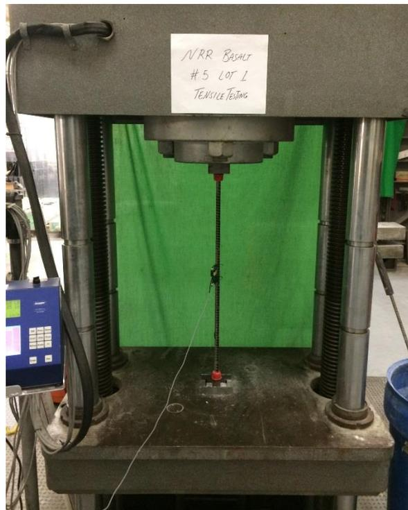
Figure 5.2 - Tensile test set-up
