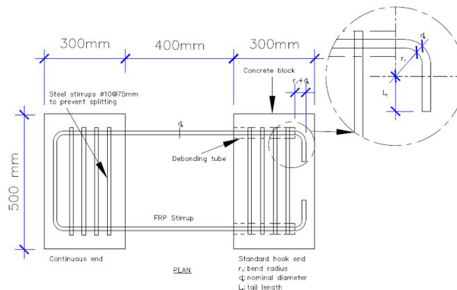
Figure 8.1 – Specimen layout for strength of bend tests.
