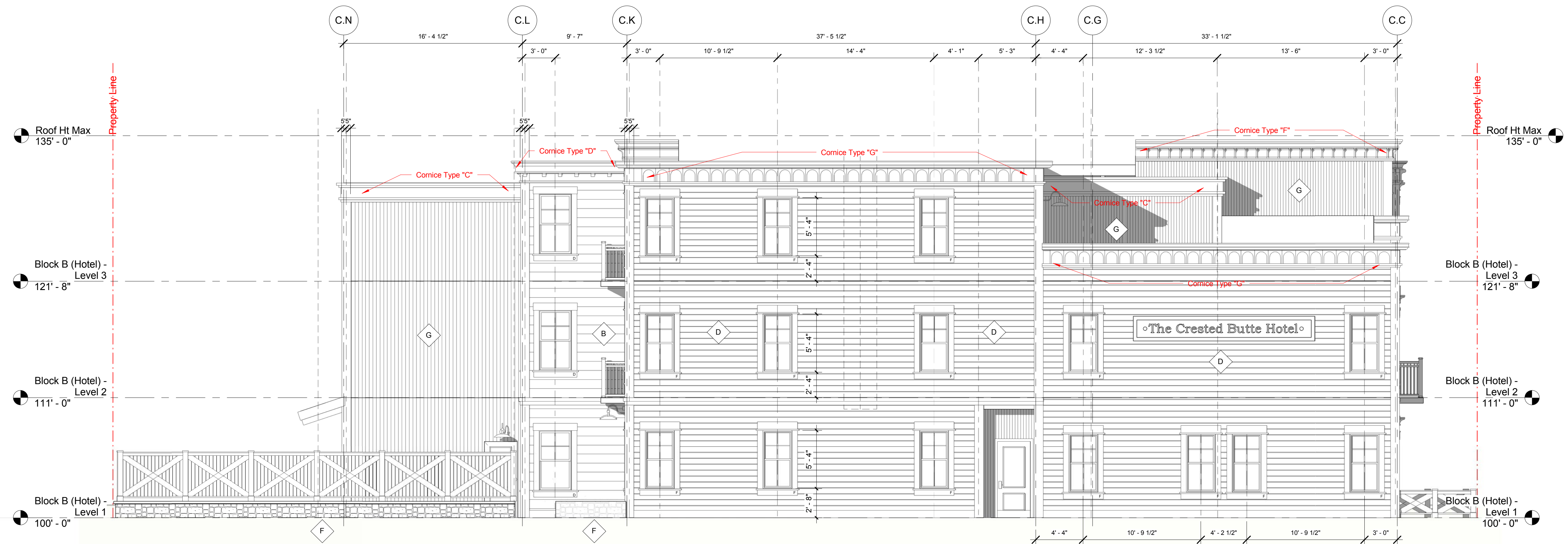
1 Annex Building - South Elevation 3/16" = 1'-0"
