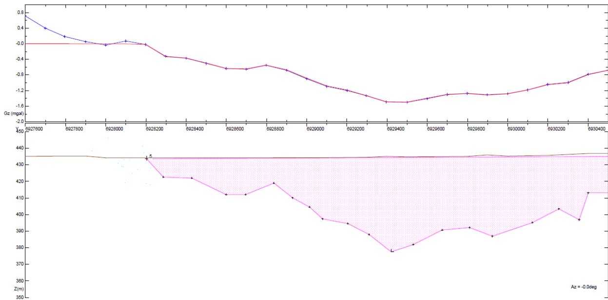
Figure 11. 2D modelling of line 340600E; the pink polygon represents channel fill with an estimated density of -0.75 \text{ g/cm}^3 relative to basement.
