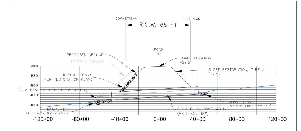
EXISTING DOWNSTREAM INVERT ELEVATION: 482.31 PROPOSED DOWNSTREAM INVERT ELEVATION: 482.65
