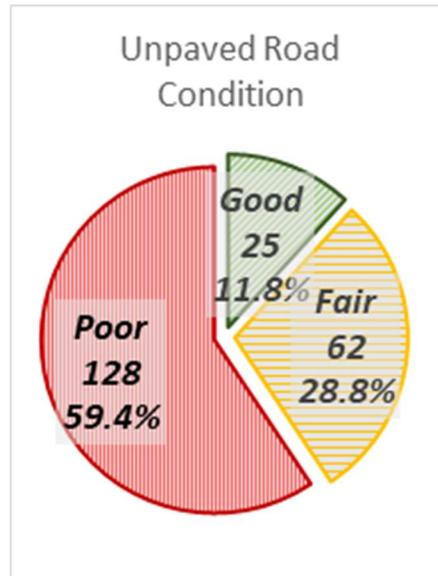
Figure 30: GCRC's 2021 unpaved road network condition by percentage of good/fair/poor
