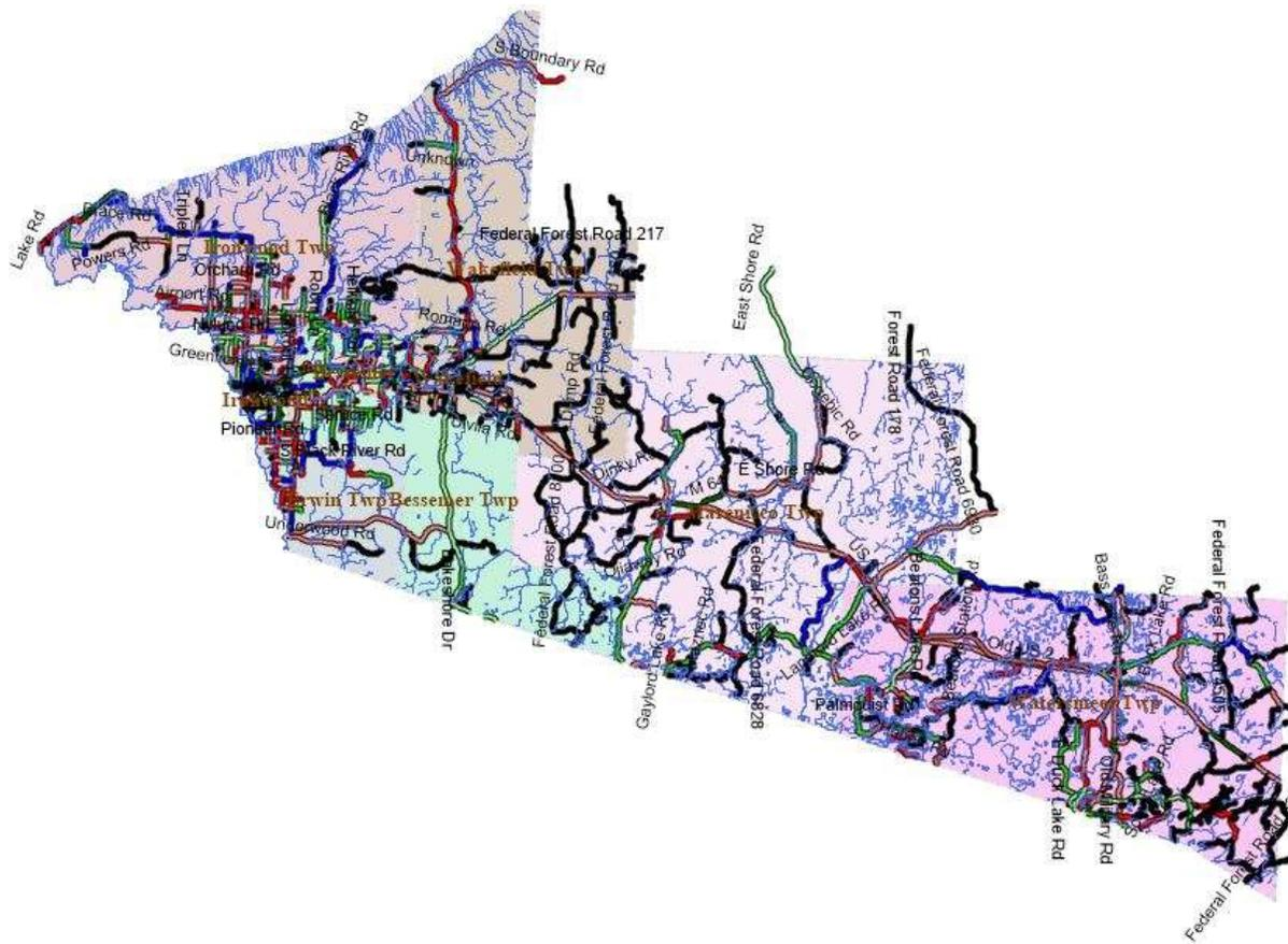
Figure 7: Map showing location of GCRC's paved roads (i.e., those managed by GCRC) and their current condition for paved roads with green for good (i.e., PASER 10, 9, 8), yellow for fair (i.e., PASER 7, 6, 5), and red for poor (i.e., PASER 4, 3, 2, 1), as well as the location of GCRC's unpaved roads in blue
