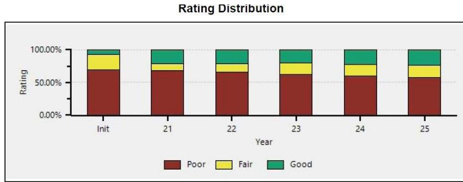
Figure 42: Forecast good/fair/poor Changes to GCRC Network Condition from planned projects on the county local paved road network.
