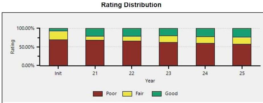
Figure 34: Forecast good/fair/poor changes to GCRC network condition from planned projects on the paved county local road network.
