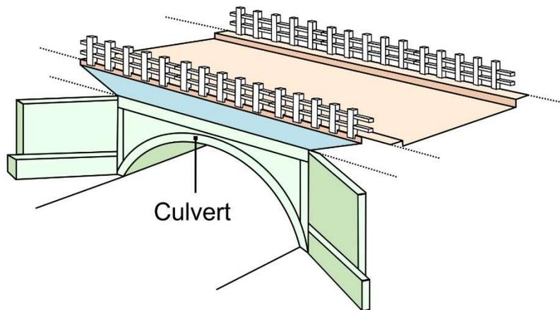
Figure C-1: Diagram of a culvert structure
