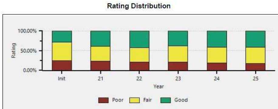
Figure 32: Forecast good/fair/poor changes to GCRC network condition from planned projects on the county primary road network.
