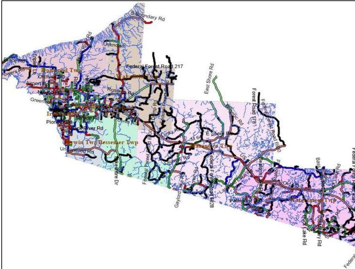
Figure 1: Map showing location of roads managed by GCRC and the current condition for paved roads in green for good (PASER 10, 9, 8), yellow for fair (PASER 7, 6, 5), and red for poor (PASER 4, 3, 2, 1) and for unpaved roads in blue
