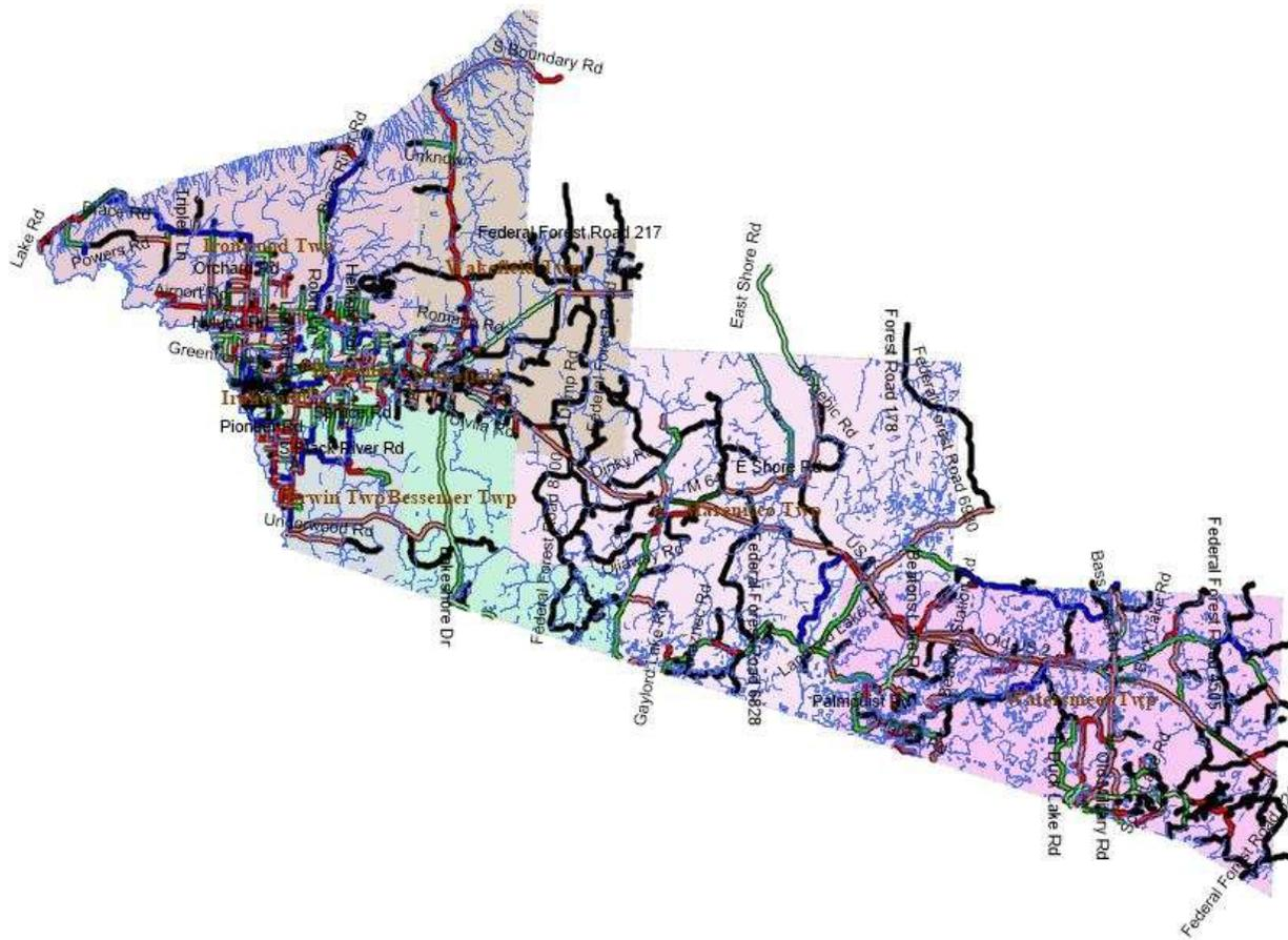
Figure 18: Map of the current paved road condition in good (PASER 10, 9, 8) shown in green, fair (PASER 7, 6, 5) shown in yellow, and poor (PASER 4, 3, 2, 1) shown in red. Only Roads owned by GCRC are shown.
