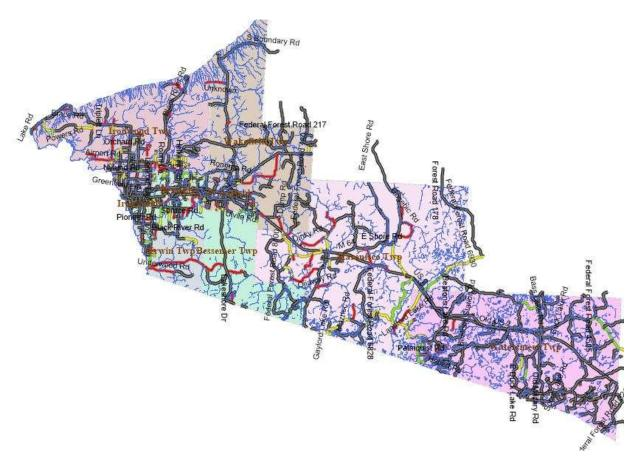
Figure 25: Map of the current IBR for surface width with good (22' and greater) shown in green, fair (16' to 21') shown in orange, and poor (15' or less) shown in red. Only unpaved roads owned by GCRC are shown.
