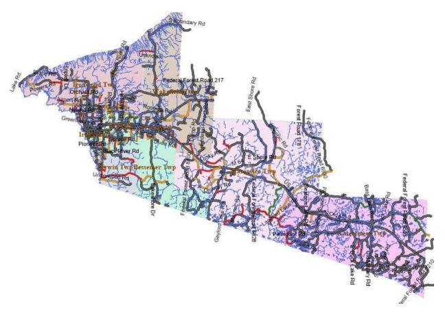
Figure 26: Map of the current IBR for drainage adequacy with good (2' or more) shown in green, fair (0.5' to less than 2') shown in orange, and poor (less than 0.5') shown in red. Only unpaved roads owned by GCRC are shown.
