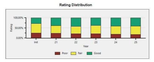
Figure 32: Forecast good/fair/poor changes to GCRC network condition from planned projects on the county primary road network.
