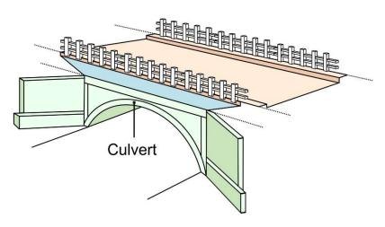
Figure C-1: Diagram of a culvert structure
