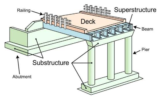
Figure 6: Diagram of basic elements of a bridge
