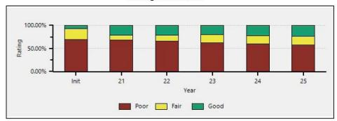
Figure 34: Forecast good/fair/poor changes to GCRC network condition from planned projects on the paved county local road network.
