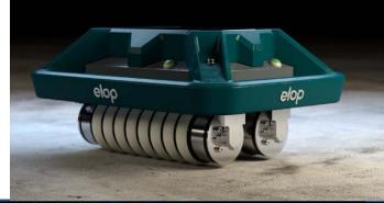
Trussbot can be fitted with any type of inspection device to map, test and record the structure of the tank. Defect parameters can be preprogramed in the software to suit the equipment specifications so the system will flag any irregularities. The camera will pinpoint any defects at a precise location, producing a map of the recorded area allowing inspection teams to interrogate the data.
