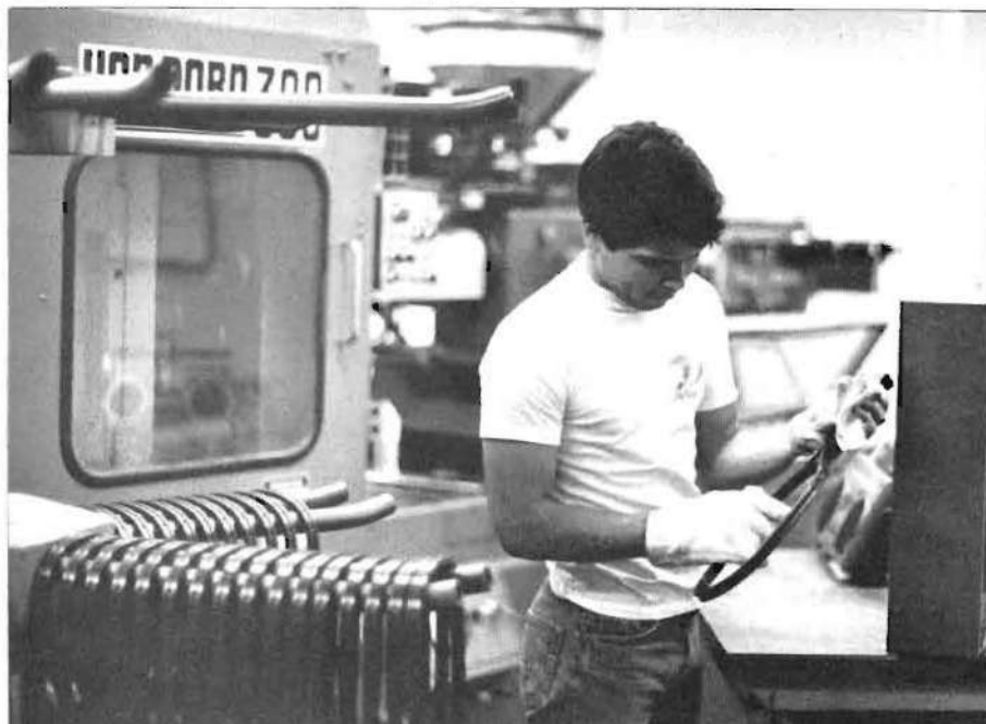
Molding racquet frames in the Richcraft factory.
