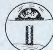
Cut-away view (showing shock absorbing action during ball contact)
