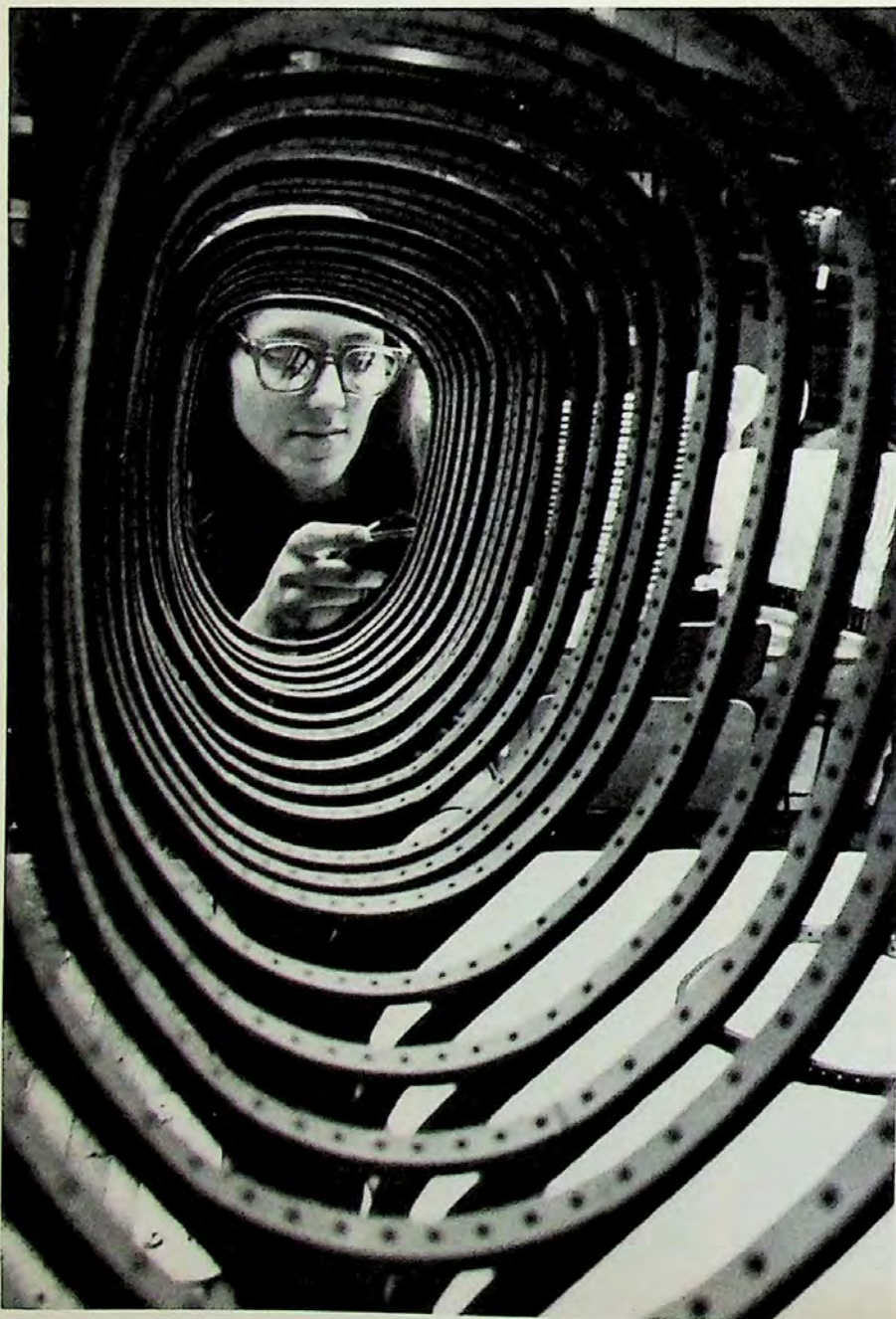
Ektelon employee Shirley Orr sands down inner walls, one of the finishing touches in making a racquet.
