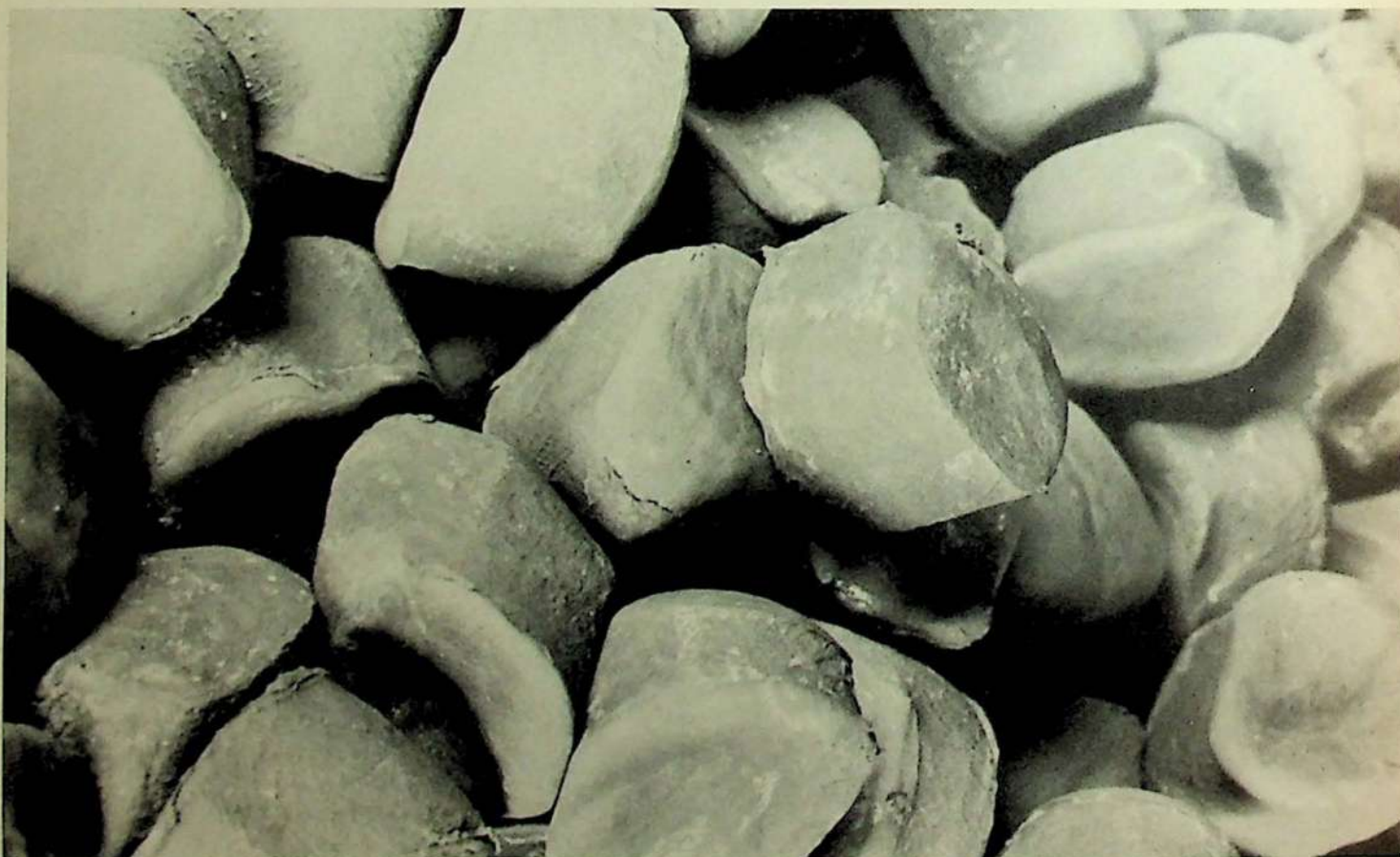
Each of these precisely weighted plugs of rubber will be dropped into a "waffle iron" mold to become half of a racquetball.
