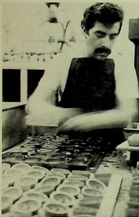
After the racquetball halves have been cut out by huge cookie cutters, they are sanded to the correct height before they are glued together.
