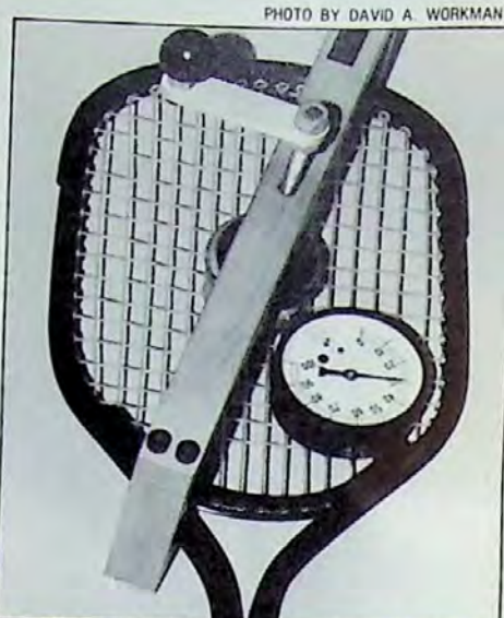
The Ski-flex tension testing device, which is used by Head and Omega to test the tension in a racquet's sweet spot.
