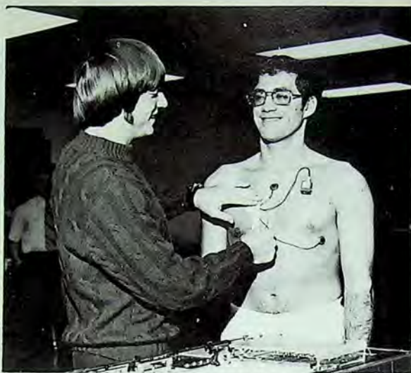
HEART RATE CAN BE MONITORED by telemetry using a small battery operated transmitter and two silver chloride electrodes. Here subject is being equipped for telemetry, prior to his handball match.
