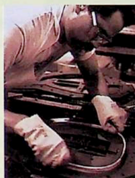
Each racquet is hand-molded, using casts forged by Ektelon's complete in-house machine and tooling department.
