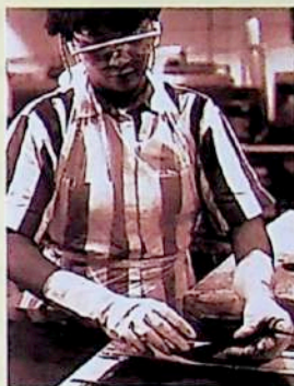
Advanced composite materials are individually layered by hand to engineering's exact specifications. Tolerances are extreme.
