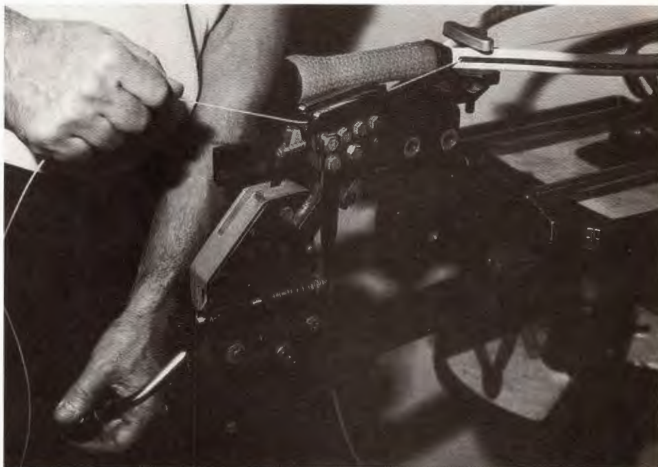
String tension is set during the stringing process by stretching the string as it's installed in the frame. String tension greatly influences the performance of the racquet. Photo: courtesy Thomas Rankin Associates, photo model: Cal Steere, Warwick, Rhode Island.
