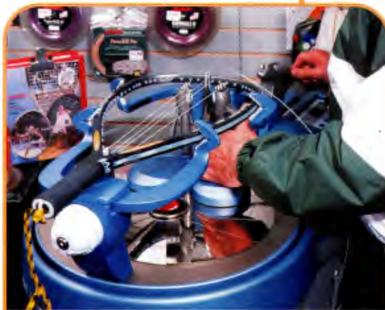
Electronic machines continuously pull the string, resulting in about 10% more tension than stringing with manual machines. Rackets strung with electronic machines also tend to hold tension better.
