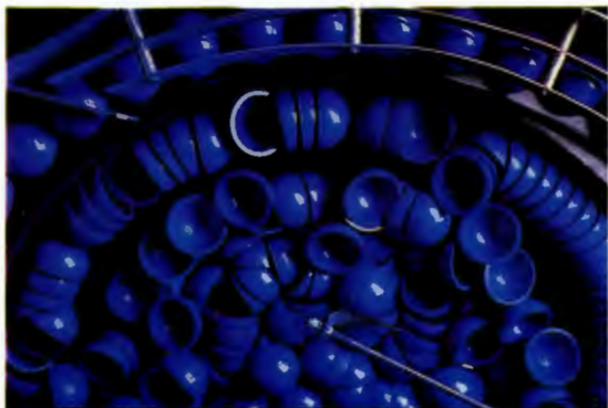
Racquetball halves lie in a vibratory feeder, preparatory to buffing and gluing of their edges. Afterwards, halves will be joined to form complete balls.
