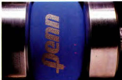
Selected racquetballs undergo repeated squeezing in a flex-tester. Each ball will withstand up to 20,000 squeezes.
