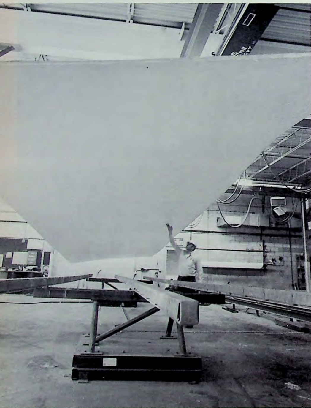
A large 10' x 45' panel as it comes from the molding machine. While panels are available in this size, other sizes—such as, 4' x 4', 4' x 8', 5' x 10', 5' x 20', or 10' x 20'—are available.
