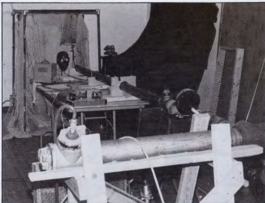
Overall view of the pneumatic apparatus used to propel racquetballs and squash balls in impact tests of eye protective devices.
