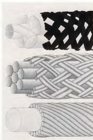
STRINGS DIFFER IN CONSTRUCTION. BOTTOM: MULTI-STRANDED MONOFILAMENT DESIGN. MIDDLE: POWERKILL™ PRO STRING, WITH ZYEX® "SEMI-MONOFILAMENT" CORE. TOP: DURAKILL™ STRING, WITH KEVLAR® MULTIFILAMENT INNER CORE AND FLATTENED SEMI-MONOFILAMENT OUTER CORE.
