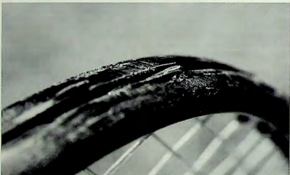
Photo 5. Bumper so worn that string is being abraded.
