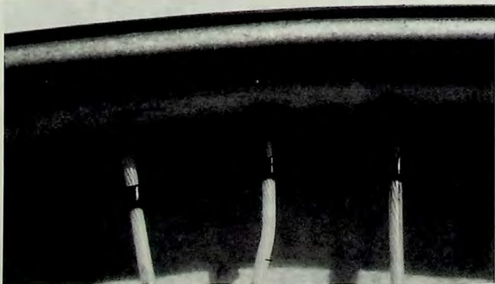
Photo 1. Grommet barrels sliced and cut away.
