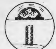
Cut-away view (showing shock absorbing action during ball contact)
