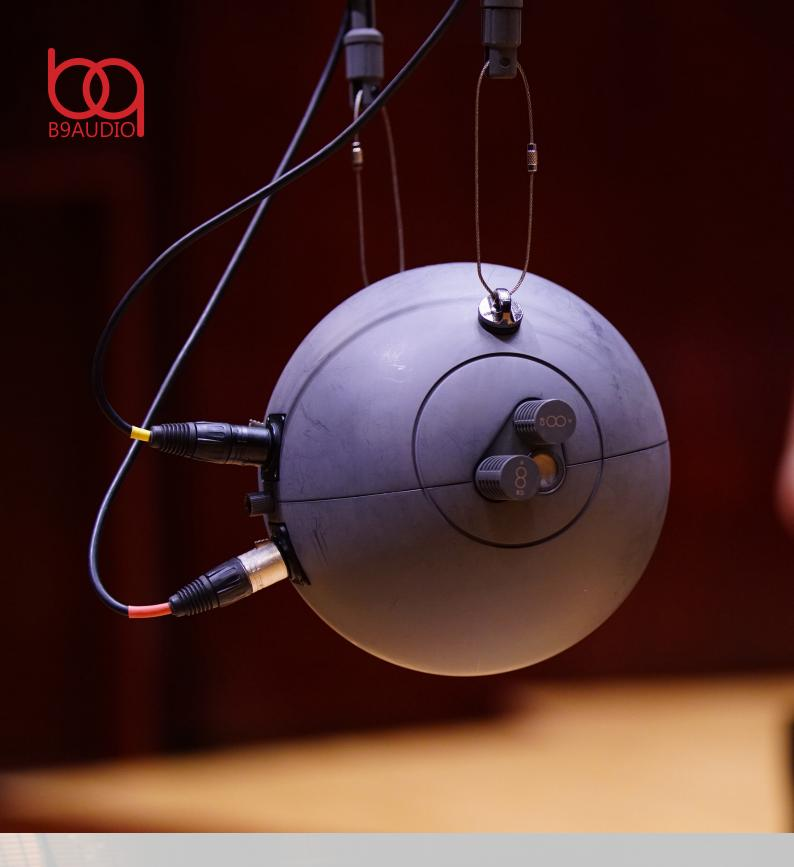
VR Ball is a binaural stereo microphone added with extra 2 pairs of figure-8 microphones in order to differentiate sound for front to back and up to down in order to decode as simple 2-channel stereo, 5.1 surround sound, or Dolby Atmos surround, and even VR sound.
