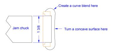
Step 8 - Detail back with 2 shallow grooves
