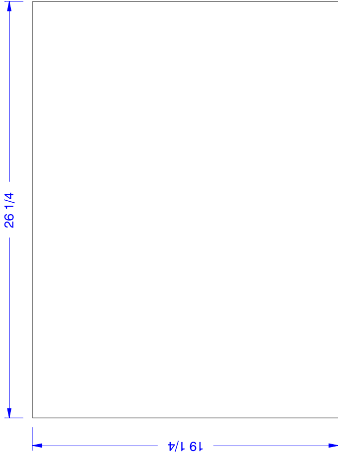
Drawer Hanger Brace - 3/4" Birch plywood
