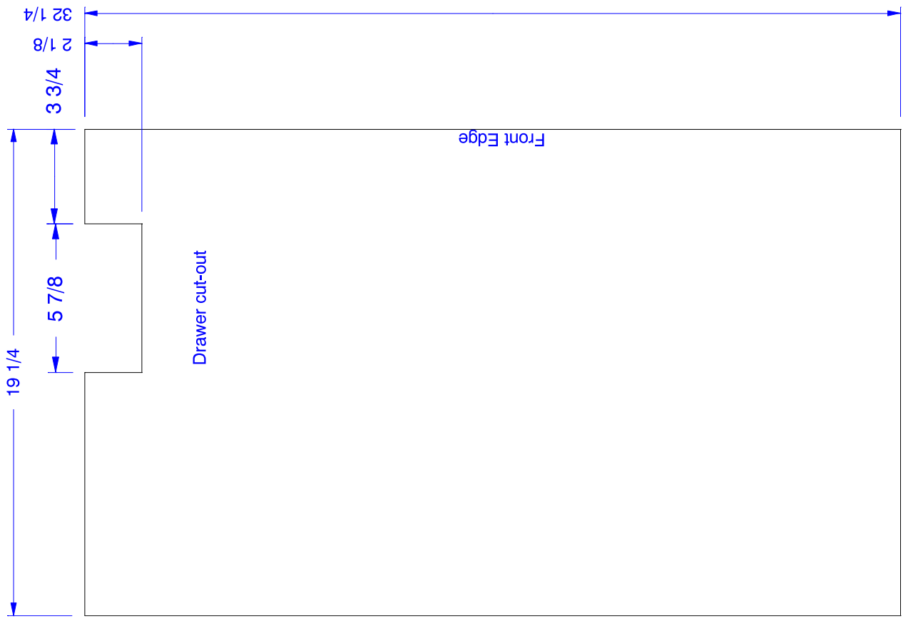
(1) Right Side Inner Panel - 3/4" Birch Plywood
