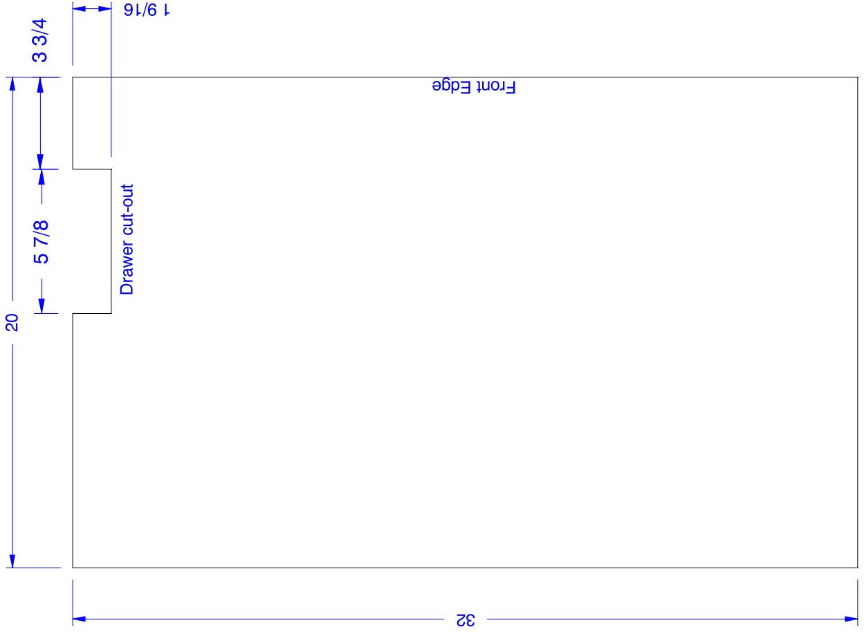
(1) Right Side Outer Panel - 1/2" Birch Plywood
