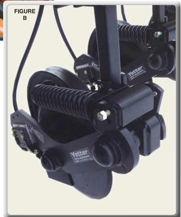
FIGURE B Viper II Unit Maximizes fertilizer placement and eliminates the problem of soil being thrown on top of plants
