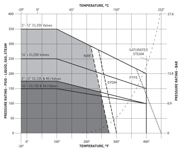
In determining field pressure ratings for Series PVIF Plug Valves that are constructed of Ductile Iron the above chart should be used. Pressure cast on valve represents maximum seating pressure; maximum hydrostatic pressure is temperature dependent, and may be higher than nominal pressure rating.
