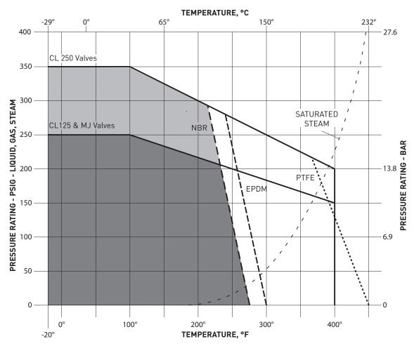
In determining field pressure ratings for Series PVII Plug Valves that are constructed of Ductile Iron the above chart should be used. Pressure cast on valve represents maximum seating pressure; maximum hydrostatic pressure is temperature dependent, and may be higher than nominal pressure rating.
