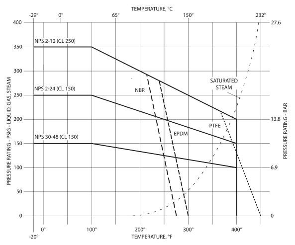
In determining field pressure ratings for Series GVI Gate Valves that are constructed of Ductile Iron the above chart should be used. Pressure cast on valve represents maximum seating pressure; maximum hydrostatic pressure is temperature dependent, and may be higher than nominal pressure rating.
