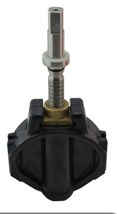
As standard all Series GVI Gate Valves feature a one-piece forged shaft with an integral thrust collar supported in both directions by replaceable permanently lubricated thrust bearings. The one-piece shaft eliminates the seal damage and leakage that often occurs with gate valves that utilize a split ring collar to retain thrust. Shafts are stainless as standard, with many options available to meet project requirements.
