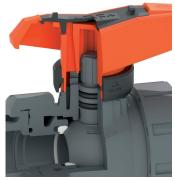
The Type 546Pro Ball Valve stem utilizes a predetermined break point oppo-site the media side of the stem seals. This break point is a groove with an inner diameter that is less than the stem seal grooves. This ensures that if there is a stem failure, the failure will occur at that point and media will not leak to the outside of the valve.
