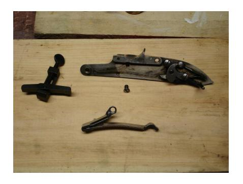
Disclaimer, if you're in a hurry, jump to slide 14. I've decided to disassemble the lock, clean and reassemble it. The Mainspring can be replaced right from this point with no further disassembly.
